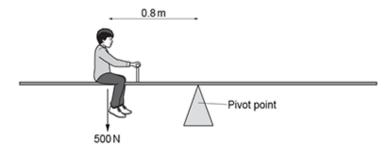
Which student will balance the see-saw when they sit on the right-hand side of the pivot point? Use the equation: moment of a force = force × distance (normal to direction of the force)
